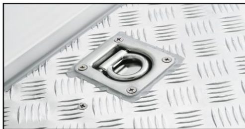
Cargo Tie Point
